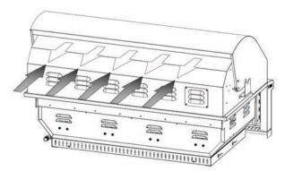
Be sure wind doesn't blow into the back of the hood gap.
