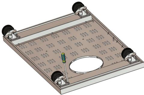
STEP-3 : Attach the Right & Left Side Panel (#3 & 4) to the Bottom Panel (#2) by using 6 sets M5x12 screw with captive washer (The tank hole of Bottom Panel#2 is on the right side.)
